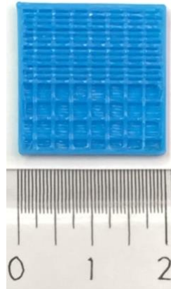
Figure 11. A 20x20mm 2 construct with 0/90° rectilinear infill (80% ID top layer, 30% ID internal layers and 100% ID bottom layer) fabricated.
