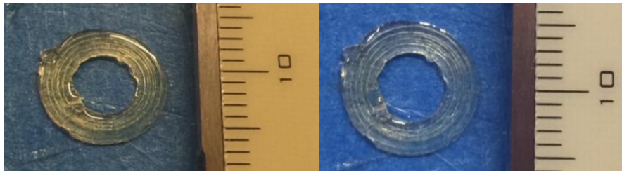
Figure 32. PLLA-Rylar-PEGDA composite disks, top view on the right shows concentric PLLA rasters and angled view on the left shows photocured Rylar-PEGDA bonded with PLLA. The disk is 10mm OD and 6mm ID with 0.4mm PLLA base (2 layers) and 0.4mm Rylar-PEGDA (2 layers) on top. Scale: 1 division=1mm.
