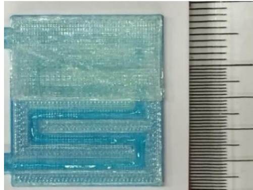
Figure 12. A 20x20mm 2 construct with a 1x1mm 2 internal channel fabricated using the FFF module and filled with toothpaste using the VE module.
